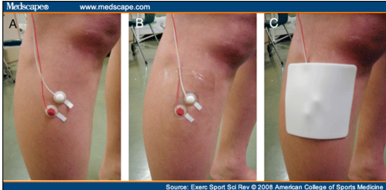
Figure 1. Waterproof dressings over each of the surface electromyography (EMG) electrodes: placed electrodes (A), covered with adhesive tape (B), and covered with foam pads (C).
