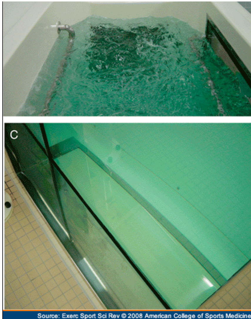
Figure 2. Side view of the flowmill (A), streaming water current (B), and underwater treadmill at the base of a water flume (C).
